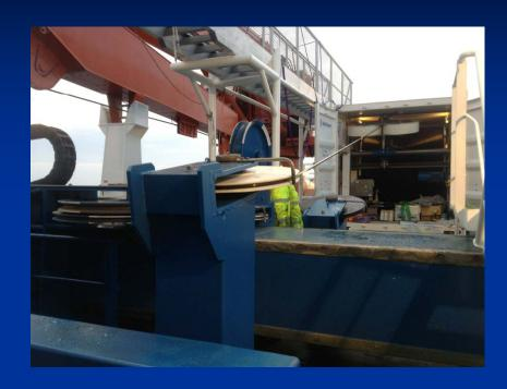
Left hand side view showing the rope run from the container over the Nylatron sheaves for deployment over the starboard Aft beam deployment system.
