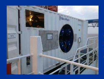
Right hand side view showing the 4 electric motors located inside the drum driving the slew ring.
