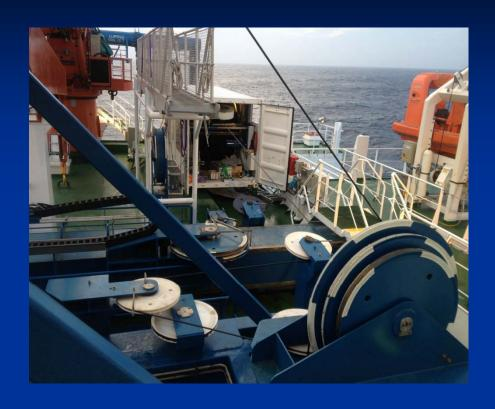
Right hand side view showing the rope run from the container over the Nylatron sheaves for deployment over the starboard forward deployment system. Left hand side view showing the rope run from the container over the Nylatron sheaves for deployment over the starboard forward deployment system.
